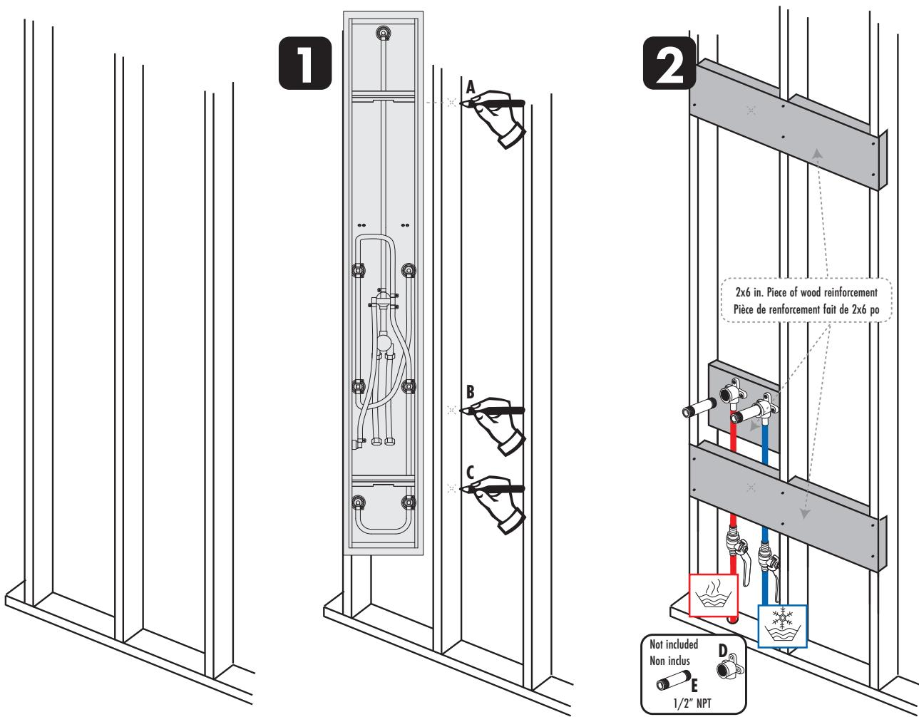
You will need to reinforce your wall with 2 x 6-inch pieces of wood as shown (2), to do this, place the shower panel against the wall at the desired height (1) to measure and mark the position of the top bracket for the 2 x 6 (A), bottom bracket position for the 2 x 6 (C), and the 2 x 6 position of the 90° drop ear elbow (B). Choose your nipples (E) to get out 3/4" (2cm) from your final wall. Provide sufficient opening at the back for easy access to connections for maintenance or repair.
