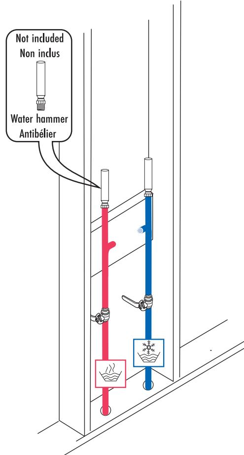
We recommend PEX or compression fittings. If welding, remove all body parts. Fittings are not included
