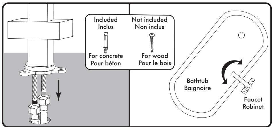
Place the base flange cover (9) on the faucet body (1) firmly tighten the base flange (11), connect the braided stainless steel hoses (8) to your water supply, and align the faucet in position. **Be careful not to damage or twist the braided hoses.**
