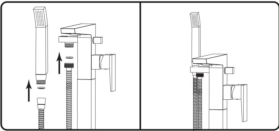
Connect flexible hoses (15) to the hand shower (13) and the faucet (1), make sure the rubber washers (14) are in place. Carefully align the threads, hand tighten firmly. **Do not use a wrench or pliers.**
