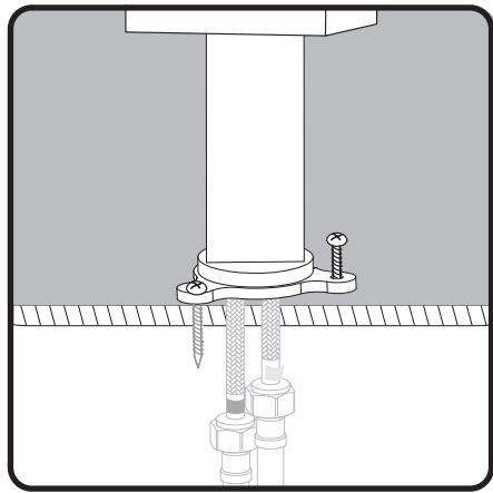
As illustrated, screw or firmly anchoring the base flange (11) firmly on the floor put in place the base flange cover (9)
