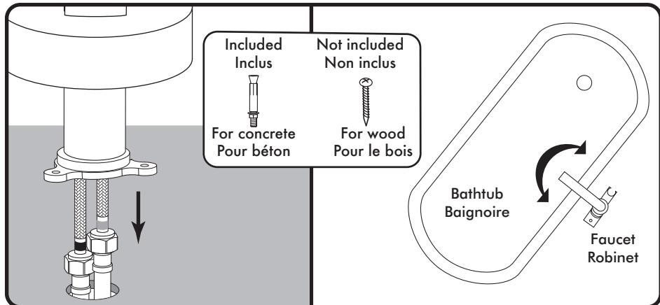
Place the base flange cover (12) on the faucet body (4) firmly tighten the base flange (14), connect the braided stainless steel hoses (11) to your water supply, and align the faucet in position. **Be careful not to damage or twist the braided hoses.**
