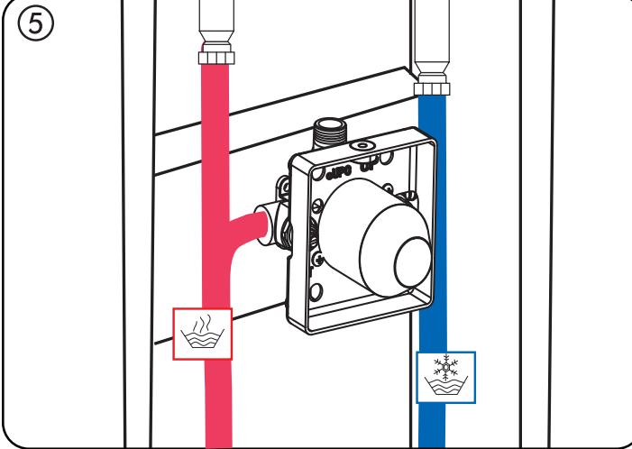
6 Testing connections. Make sure the connections are watertight by slowly opening the water supply. In case of a leak, shut off the water supply and tighten connectors with the appropriate tool.
