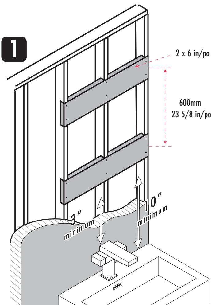
Determine the height of your medicine cabinet. The bottom should be at least 3 in. from the faucet and 10 inches from the sink. To secure the installation, you will need to reinforce your wall with a 2 x 6 in. wood stud or a 1/2 in. plywood panel covering at least 3 posts. The stud should have a maximum spacing of 16 in.
