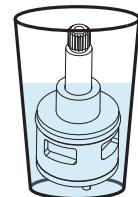
If a cartridge is not responding well, you will need to clean it in a solution of half vinegar and half hot water, ideally overnight. Make sure it turns easily, then brush and rinse it with clean water. Apply plumbing grease to the O-rings and put the cartridge back into place. Remember to manipulate the handle of the thermostatic valve knob once a month and two or three times in a row to avoid limescale fixation and have your cartridges cleaned if necessary.
