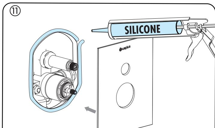
Apply silicone to prevent infiltration into the wall.
