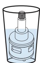
If a cartridge does not respond well, you will need to clean it in a solution of half vinegar and half hot water, ideally overnight. Brush and then rinse it under clean water. Apply plumbing grease to the O-rings before replacing the cartridge.
