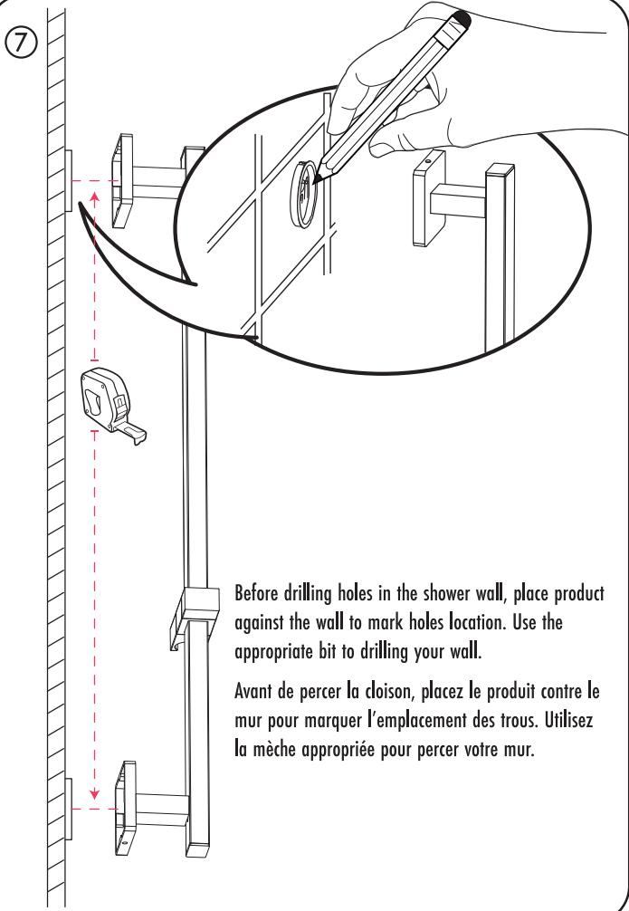
Before drilling holes in the shower wall, place product against the wall to mark holes location. Use the appropriate bit to drilling your wall.
