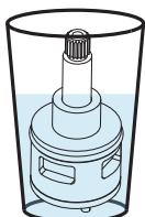
If a cartridge does not respond well, you will need to clean it in a solution of half vinegar and half hot water, ideally overnight, brush and then rinse it under clean water. Apply plumbing grease to the O-rings, replace the cartridge. Align the colored lines for a thermostatic cartridge or adjust if necessary.
