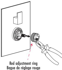
If the water is not hot enough, you can remove the pressure balance cartridge's temperature O-Ring to loosen the temperature control. Although, doing so would go against ASME's anti-scalding standards.
