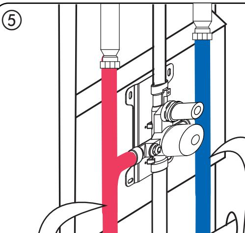
You will need to fix the pipes securely to avoid water hammer.
