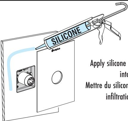
Apply silicone to prevent infiltration into the wall.
