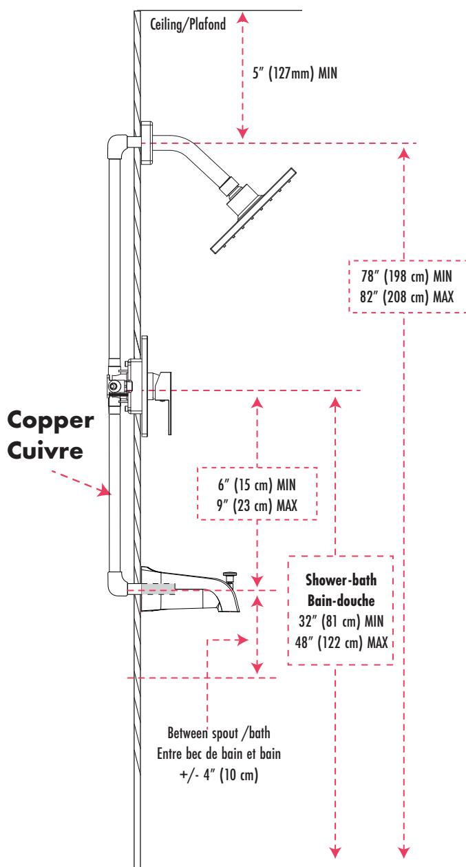
The use of copper tubing to connect the valve to the bathtub spout **IS MANDATORY**. Do not use PEX type pipes or a quick connect this could cause a flow restriction and backflow to the shower. We cannot be held responsible in the event of an incident related to an installation that does not take this advice into account.
