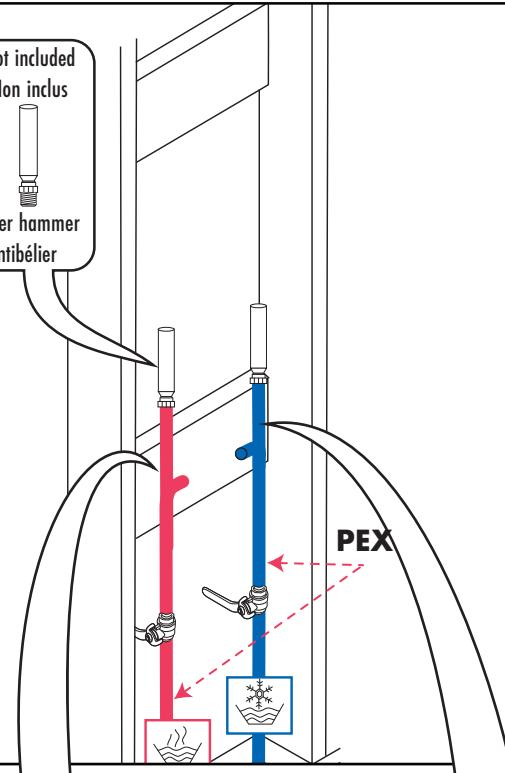
You will need to fix the pipes securely to avoid water hammer.
