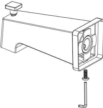
Use of copper pipe for installing the valve on the bathtub spout **IS MANDATORY**. Pipes with PEX, Wirsbo, HeatLink and other types of fittings may cause flow restriction and backflow to the shower. We will not be held responsible for any damages to an installation that does not comply with above guidelines.
