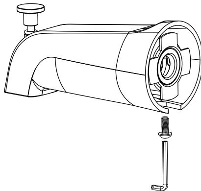
Use of copper pipe for installing the valve on the bathtub spout **IS MANDATORY**. Pipes with PEX, Wirbo, HeatLink and other types of fittings may cause flow restriction and backflow to the shower. We will not be held responsible for any damages to an installation that does not comply with above guidelines.
