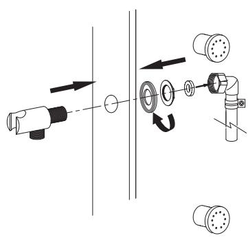
Put on the impurity filter washer (A). Apply teflon (B) tape to the pipe nipples. Install the 90° connectors firmly on the pipe nipples and tighten with 1/4 turn with an adjustable wrench. Connect the hoses to the shower panel while making sure they are not twisted. Install the shower panel on the wall brackets. It is recommended not to apply silicone seal around the panel. **IT IS FORBIDDEN** to connect the flexible hoses inside the walls.
