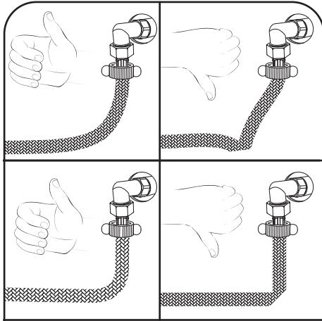
If a hose is bent, the thermostatic cartridge will not work properly.
