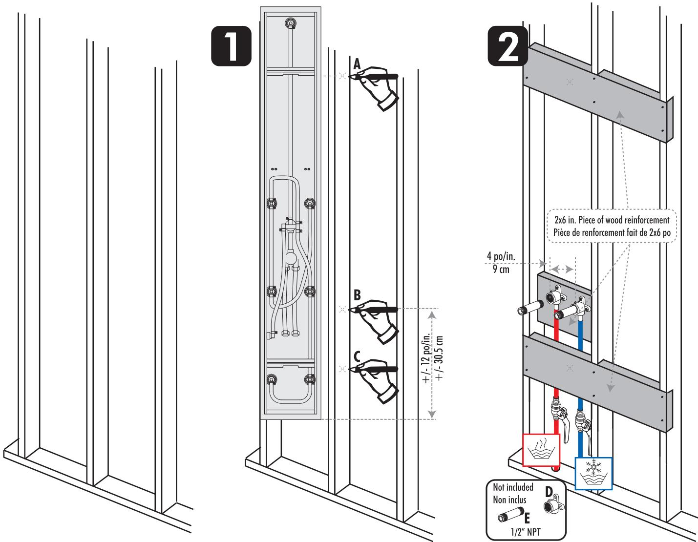
You will need to reinforce your wall with 2 x 6 inches pieces of wood as shown (2), to do this, place the shower panel against the wall at the desired height (1) to measure and mark the position of the top bracket for the 2 x 6 (A), bottom bracket position for the 2 x 6 (C), and the 2 x 6 position of the 90° drop ear elbow (B). Choose your nipples (E) to get out 3/4 " (2cm) from your final wall. Provide sufficient opening at the back for easy access to connections for maintenance or repair.
