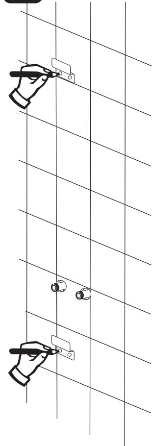
Locate your 2x6. Place and mark the position if the wall bracket at the correct position.
