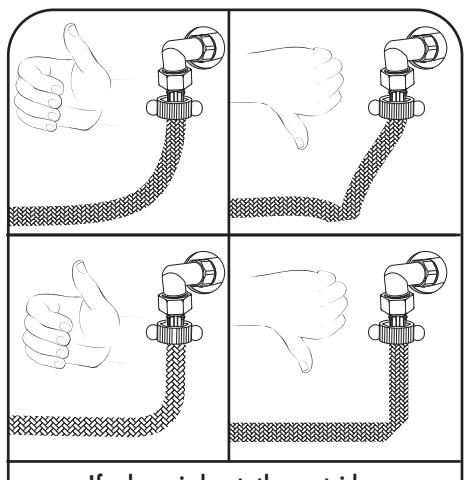
If a hose is bent, the cartridge will not work properly.
