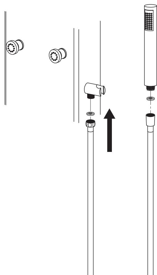
Put on the impurity filter washer (A). Apply teflon (B) tape on thread. Install the 90° (if necessary) by screwing them in firmly by hand and tighten with 1/4 turn with an adjustable wrench. Connect the hoses to the shower panel while making sure they are not twisted. Install the shower panel on the wall brackets. It is recommended not to apply silicone seal around the panel. **IT IS FORBIDDEN** to connect the flexible hoses inside the walls.
