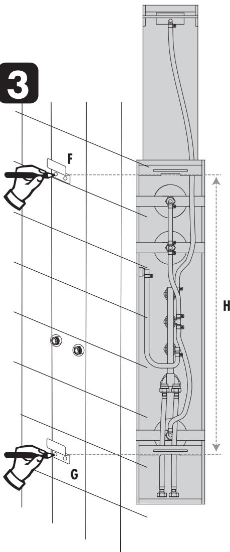
Place and mark the upper shower panel bracket (F), measure the distance between the both shower panel brackets (H) in order to place and mark at the right position the support of the bottom (G).
