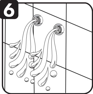
Turn on the faucet and leave the water running for at least one minute to evacuate the air and dirt trapped in the pipes.
