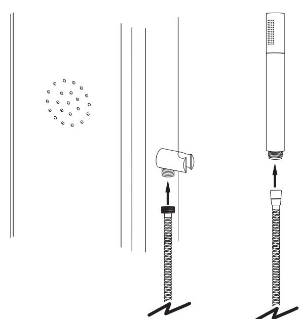
Put on the impurity filter washer (A). Apply teflon (B) tape on thread. Install the 90° (if necessary) by screwing them in firmly by hand and tighten with 1/4 turn with an adjustable wrench. Connect the hoses to the shower panel while making sure they are not twisted. Install the shower panel on the wall brackets. It is recommended not to apply silicone seal around the panel. **IT IS FORBIDDEN** to connect the flexible hoses inside the walls.
