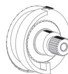
When you reinstalling the temperature adjustment gasket, place color (red or white) in a straight line.
