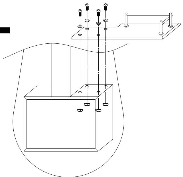
Before installing the panel, check to make sure your water supply pipes are located where a part of the panel will fastened. Your water supply should be located at least 23 5/8 in. from the floor.
