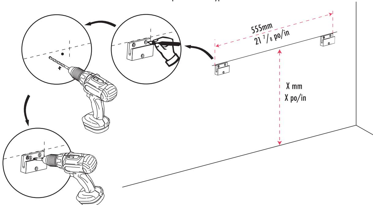
Install water ducts and drainage system as required for your sink model. Make sure that these do not interfere with the elements of your piece of furniture. Hang your furniture on the wall. Make sure the brackets are properly seated.
